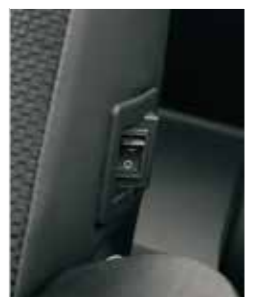
Seat heater switch
